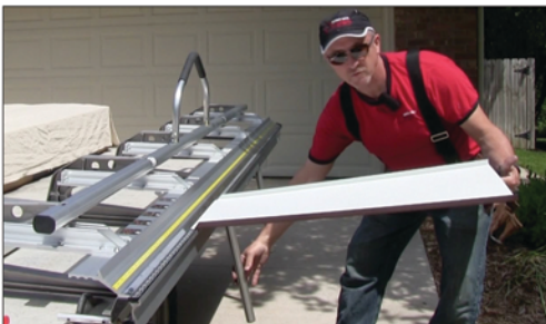
Bend the tabs up slightly past 90°
